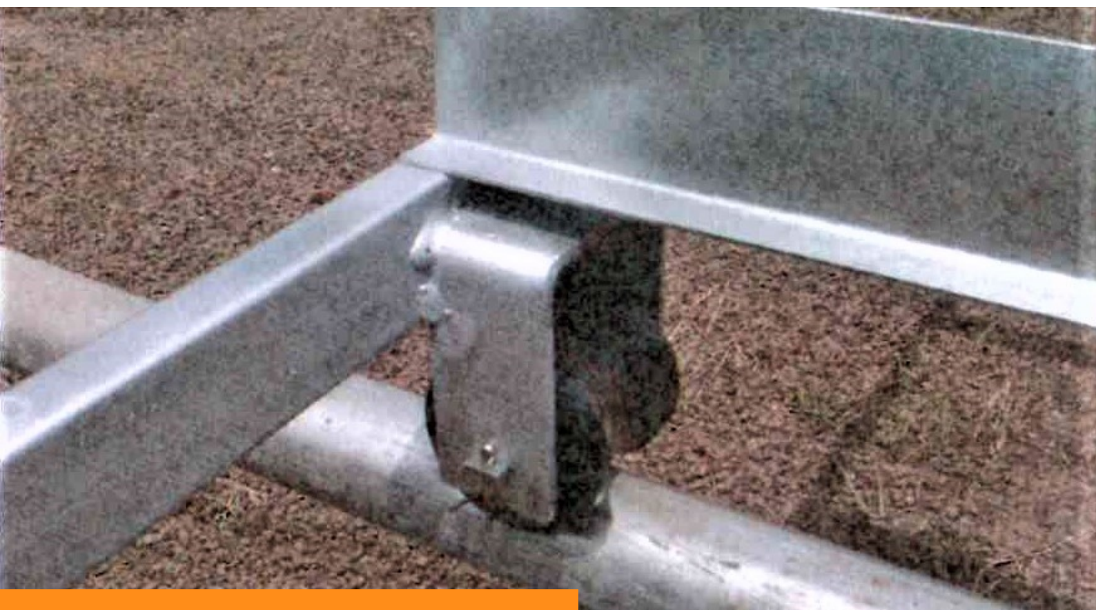
TRAYS MOVED ON/OFF BENCHES USING "T" BAR GUIDES (ABOVE) ON WILLIAMES "T" ROLLING BENCHES (BELOW)
