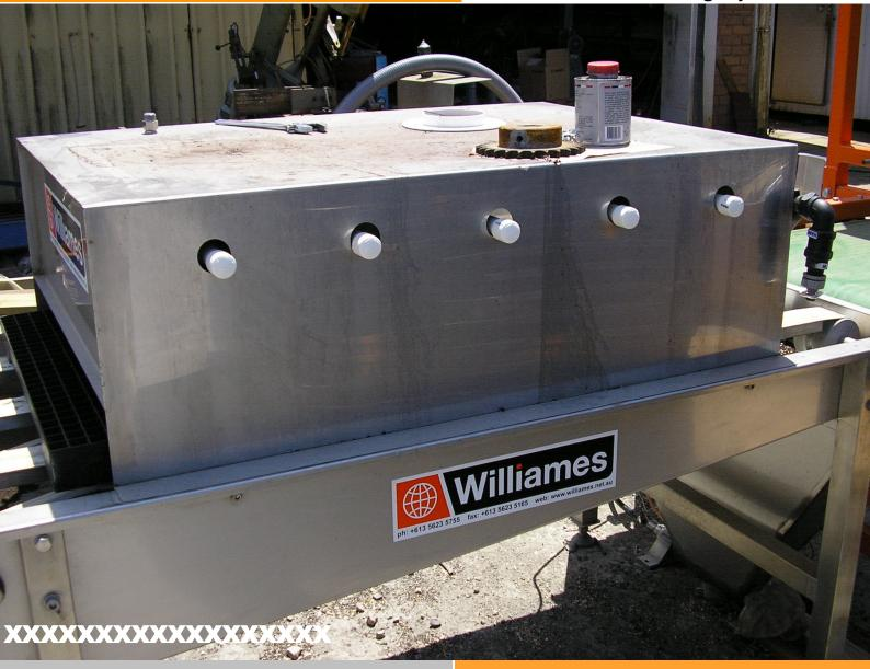
The Williames DC WIDE WATERING TUNNEL waters the tray after it has been filled, seeded and covered.
